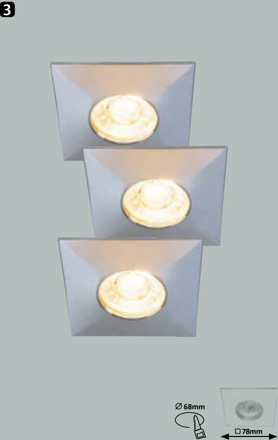
2 I078 P • LED / 4W (350lm, 3000K) incl. IP20/IP44 white
